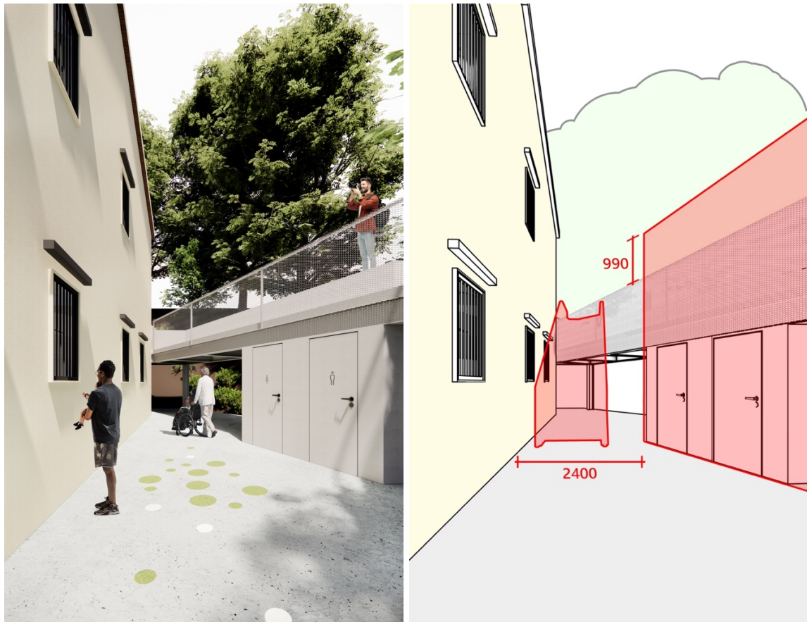
Figure 13. Comparison between the new fire escape staircase and toilet block (base drawing) and the existing staircase and the existing toilet block (outlined in red)
